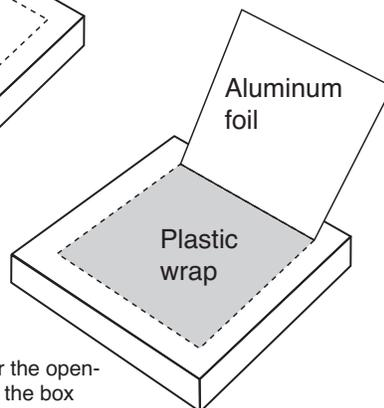
4. Measure a piece of plastic to fit over the opening you created by forming the flap in your pizza box. The plastic should be cut larger than the opening so that it can be taped to the underside of the box top. Be sure the plastic becomes a tightly sealed window so that the air cannot escape from the oven interior.
