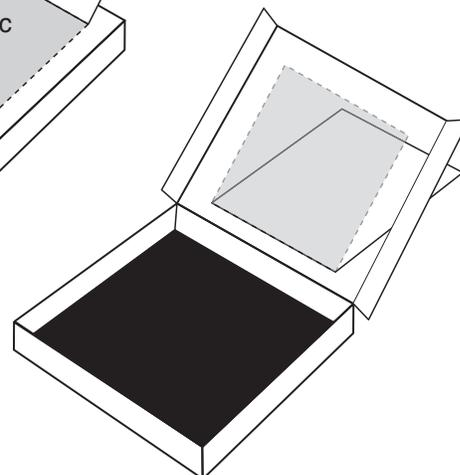
5. Cut another piece of aluminum foil to line the bottom of the pizza box and carefully glue into place.
